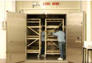
The High/Low Temperature Walk-in Treatment Chamber
