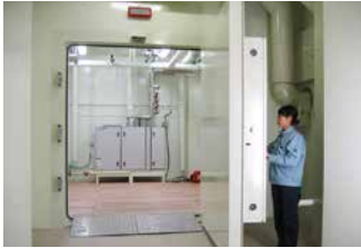
A Multi-functional Fumigation Chamber Capable of Carbon Dioxide and Low Oxygen Concentration Treatments
