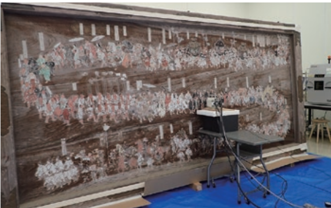
Examination Using X-ray Fluorescence Spectrometer
