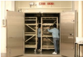
The High/Low Temperature Walk-in Treatment Chamber
