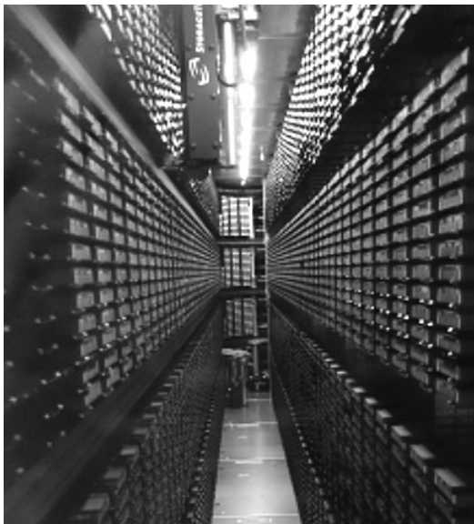
A large-scale digital repository using magnetic tape technology for motion pictures (Photo by author, Los Angeles, April 3rd, 2015)
